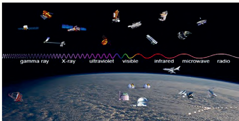
Figure 1.4 Detection of different components of electromagnetic radiation by telescope
