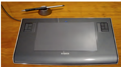
Figure 4.17 A tablet with a specially designed pen to write with is another application of magnetic induction.
